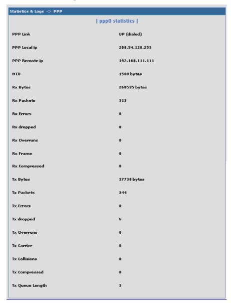
This is an example of the PPP Statistics & Logs screen. It shows PPP statistics when PPP is enabled.
